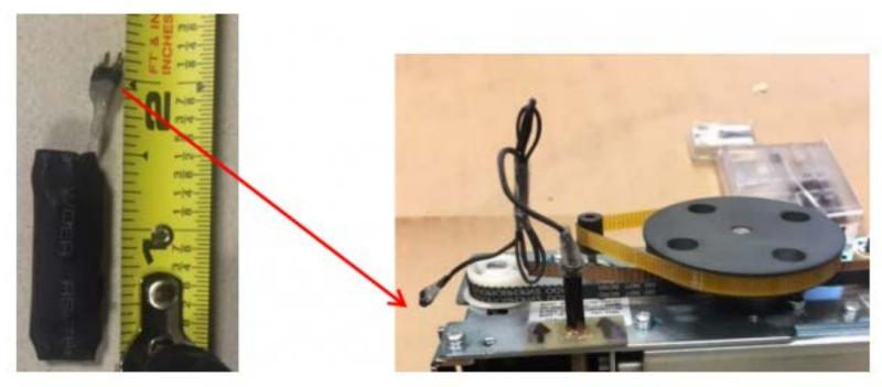
At left, the skimming control device. Pictured right is the skimming control device with wires protruding from the periscope. These were recovered from a cash machine in Connecticut.
